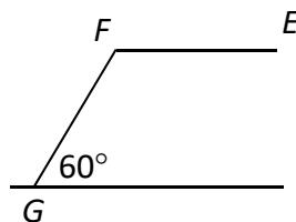
The rod  $FE$  is horizontal, and the rod  $GF$  is inclined at an angle of  $60^\circ$  to the horizontal.  $G$  is on the point of slipping.
