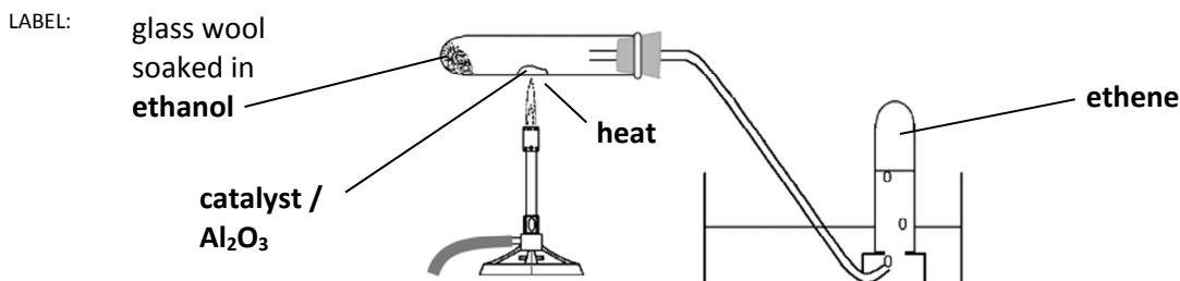
[Locations of ethanol, ethene, catalyst ( $Al_2O_3$ ) must be labelled;
